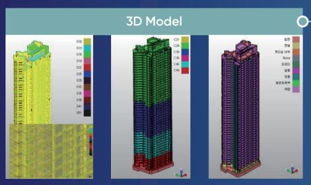
Concrete View By Strength Formwork View By Type Rebar View By Dia
